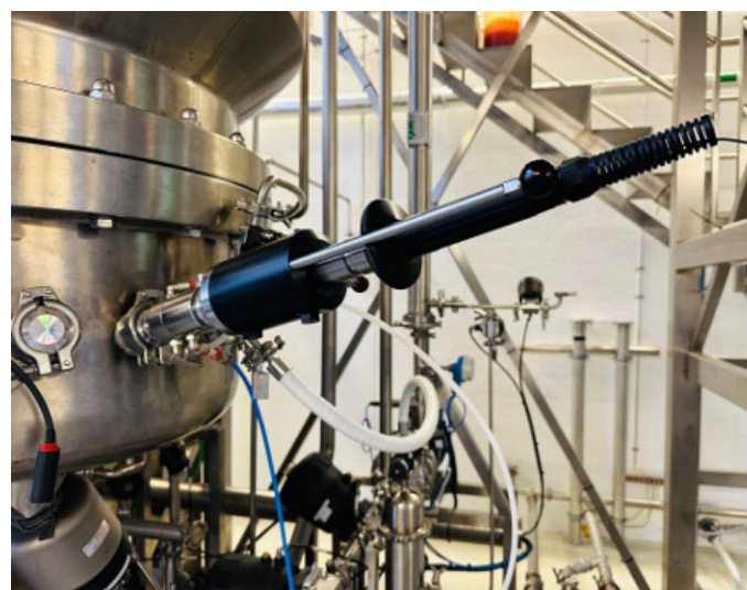
Figure 2: Unisense H_2 sensor mounted in retractable housing on 150 L fermenter
