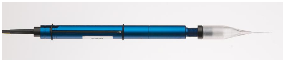
Figure 4: Redox microselectrode in the Microrespiration guide.
