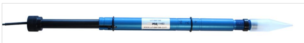
Figure 3: Microsensor mounted in the Microrespiration guide.
