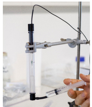
Injecting calibration liquid into protection tube using the calibration cap.
