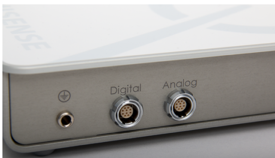
Figure 5: Connectors for Digital and Analog in and output and for the grounding cable (left).
