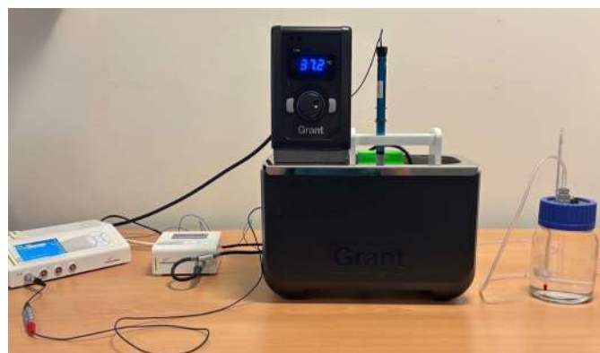
Figure 1: MicroRespiration setup showing the sample chambers submerged in a water bath.
