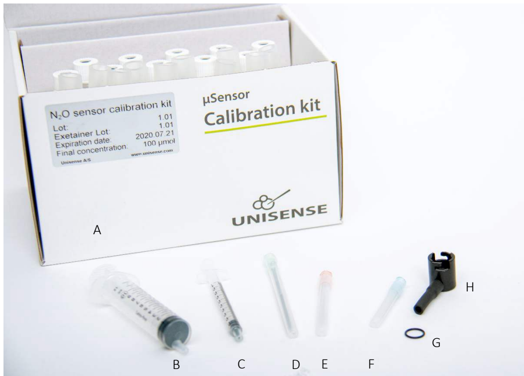
Figure 1: Calibration kit contents: A: Calibration kit box with Exetainers and ampoules, B: 10 ml syringe, C: 1 ml syringe, 0.5 ml Syringe, D: 80 x 2.1 mm needle (green), E: 50 x 1.2 mm needle (red), F: 30 x 0.6 mm needle (blue), G: O-ring, H: Calibration Cap with tubing.
