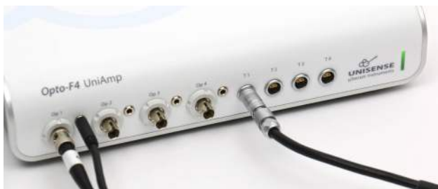
The MicroOptode and temperature sensor connected to the Opto-F4 UniAmp
