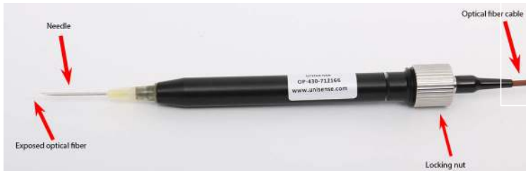
MicroOptode with its components
