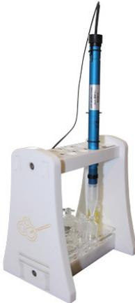
The MR2-Rack holds both the MR-Sensor/s and MR-Chambers so the sensor can easily be placed into the chamber. The MR2-Rack has magnetic stirring controlled by the MR2-Stirrer Controller.
