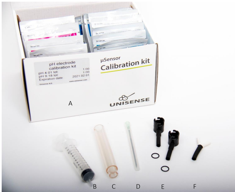
Figure 1: Calibration kit contents: A: Calibration kit box with pH buffer pouches, B: 10 ml syringe, C: 10 cm tube for reference electrode, D: 80 x 2.1 mm needle (green), E: two Calibration Caps with tubing and O-rings, F: Y-connector with tubing.
