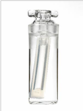
Figure 5: Zero calibration chamber (MR-Ch 0-calibration). The zero solution is outside the silicone tubing and pure water is inside. The oxygen in the water inside the tubing diffuses through the silicone tubing into the zero solution where it is consumed.
