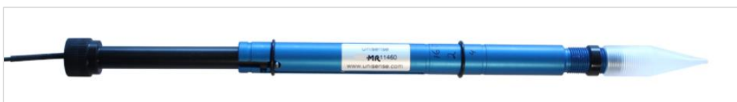
Figure 3: Microsensor mounted in the Microrespiration guide.
