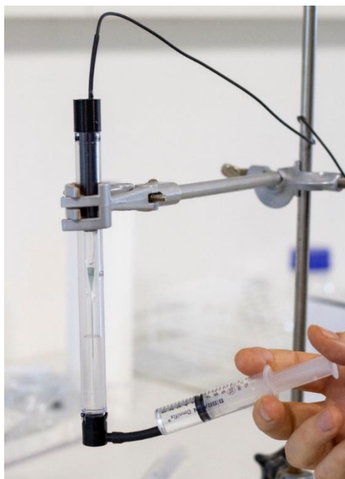
Figure 2: Sulfide sensor with the calibration cap mounted. Calibration solution is injected with the 10 ml syringe.
