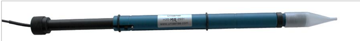
Figure 3: H 2 S sensor in the Microrespiration guide.
