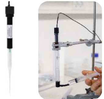
SULF-Sensor Injecting calibration liquid into protection tube using the calibration cap.
