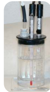
CAL300 with microsensors and bubbling with air.
