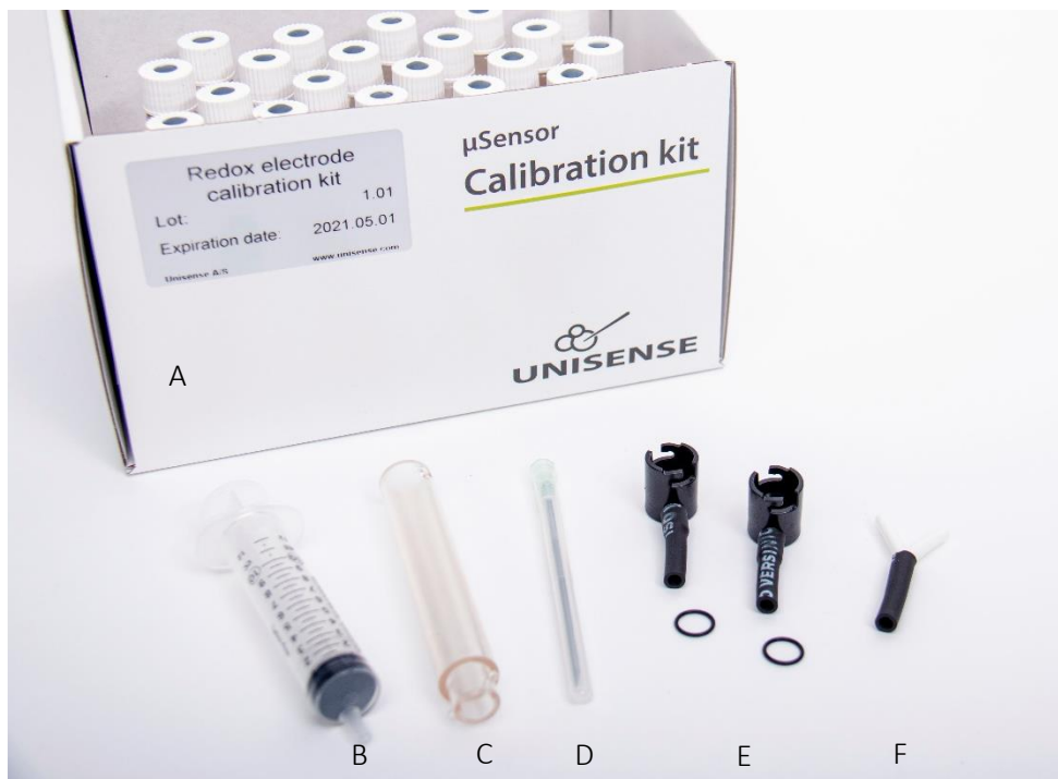
Figure 1: Calibration kit contents: A: Calibration kit box with Exetainers, B: 10 ml syringe, C: 10 cm tube for reference electrode, D: 80 x 2.1 mm needle (green), E: two Calibration Caps with tubing and O-rings, F: Y-connector with tubing.
