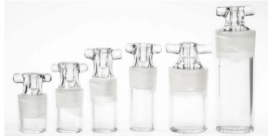
Chambers: Small (400-4000 \mu L) Medium (20, 40 and 50 mL) Large (200-400 mL)
