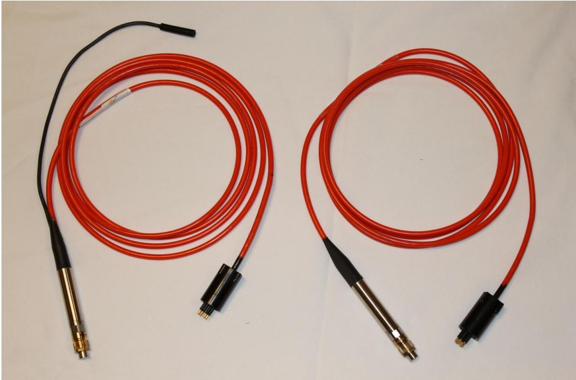
*In situ amplifier unis, left: potentiometric (e.g. pH, redox), right: amperometric (e.g. O<sub>2</sub>, H<sub>2</sub>S).*
