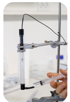
Injecting calibration liquid into protection tube using the calibration cap.
