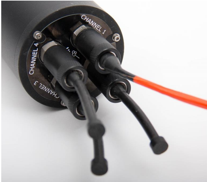
Figure 1: Four channel FDL Mini seen from the sensor connector end. An In Situ UniAmp amplifier is plugged into channel 1 and channels 2-4 are closed with dummy plugs.
