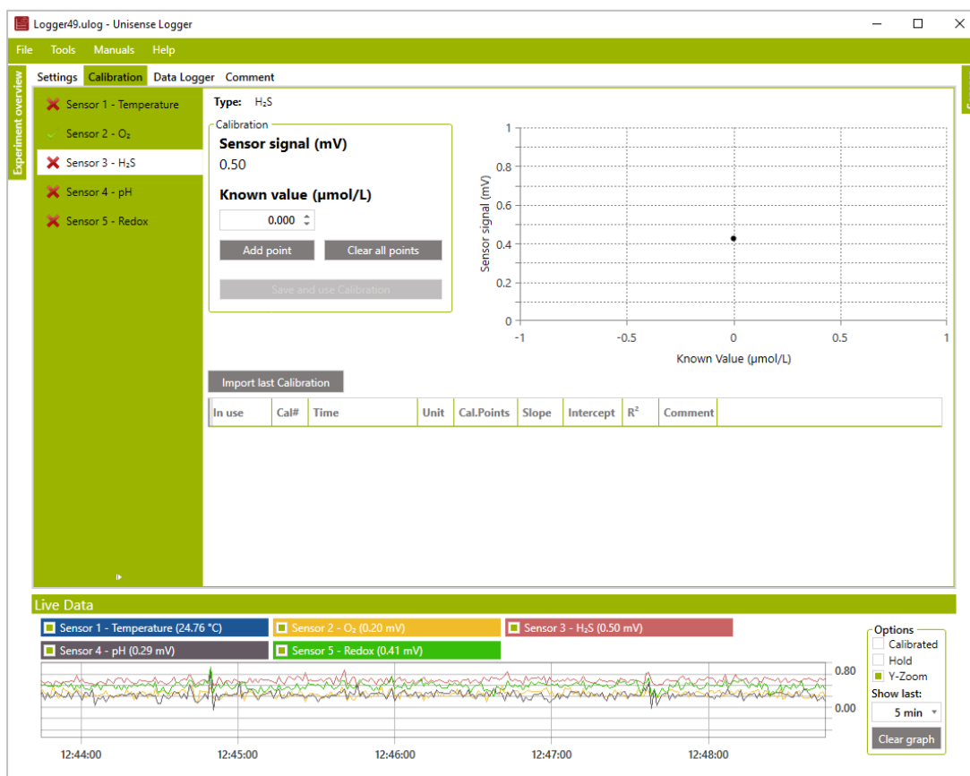
Figure 11: The Calibration window in SensorTrace Logger. The live data from all sensors can be seen in the “Live Data” frame at the bottom of the window. Most Unisense sensors require a 2-point calibration, zero and one known concentration. To record a calibration point, expose the sensor to a known concentration, enter this in the “Known value ( \mu\text{mol/L} )” box, let the sensor stabilize, and click “Add point”. Repeat this for the second calibration point. Click “Save and use Calibration” to save the calibration.
