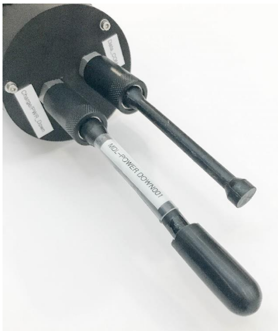
FDL Mini with Off-dongle and dummy mounted at the non-sensor end (left). Off-dongle (right)
