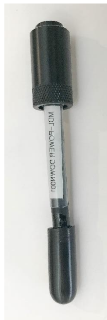
FDL Mini with Off-dongle and dummy mounted at the non-sensor end (left). Off-dongle (right)
