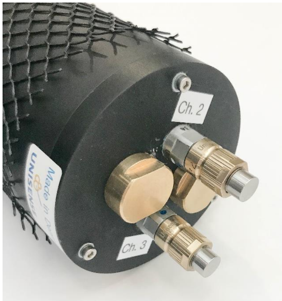
Two channel (left) and four channel (right) FDL Mini seen from the sensor end. These dataloggers are with built in amplifiers.
