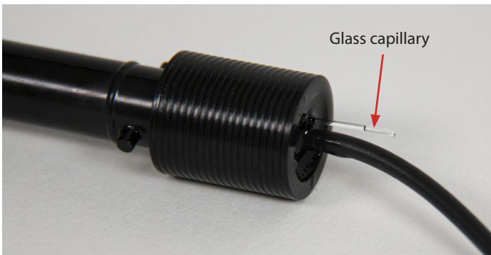
Figure 4: Detailed view of the top of the sensor shaft showing the glass capillary that should be broken off before use.
