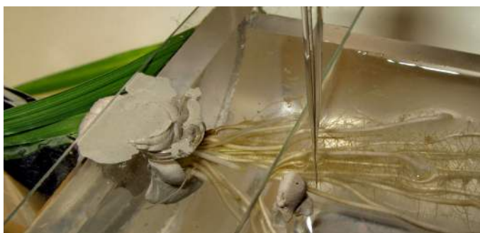
Laboratory setup with double chamber, the sensor is positioned into root cortex. Photo: Ole Pedersen
