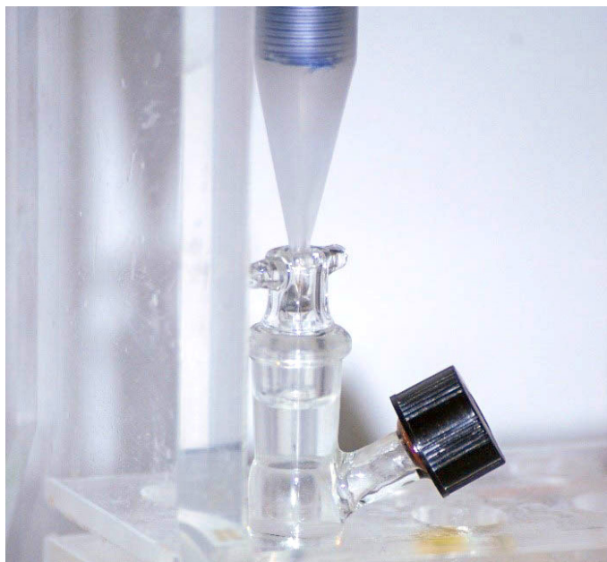
Figure 1: MicroRespiration setup showing a Unisense oxygen microsensor (OX-MR) inserted into a MicroRespiration glass chamber containing the 4T1 cells. The different substrates were injected through the rubber cup with a Hamilton syringe.
