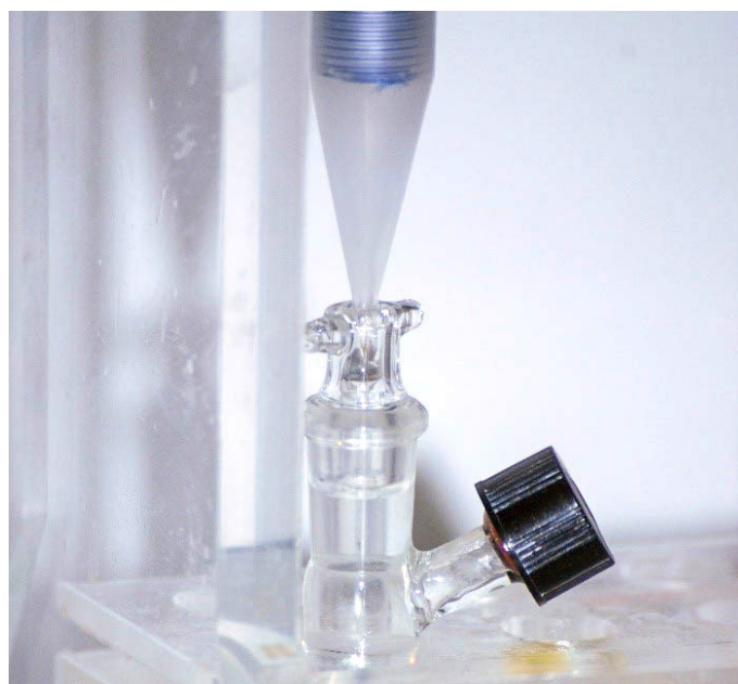
Figure 1: MicroRespiration setup showing a Unisense oxygen microsensor (OX-MR) inserted into a MicroRespiration glass chamber containing the 4T1 cells. The different substrates were injected through the rubber cup with a Hamilton syringe.
