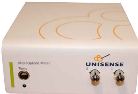
Front view of MicroOptode Meter
