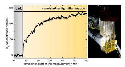
**Figure 1.** *Microsensor measurement of the* H<sub>2</sub> *produced when the sample was illuminated with sunlight (left).* H<sub>2</sub>-NPLR microsensor in the cuvette containing the active semiconducting material (orange substrate) and water (right).
