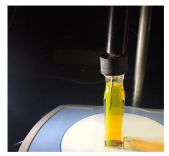
**Figure 2.** *H*<sub>2</sub> generation over time measured with the Unisense H2-NPLR microsensor (left) and experimental setup showing the hydrogen microsensor pierced through the lid into the sample measuring the H<sub>2</sub> generation (above).
