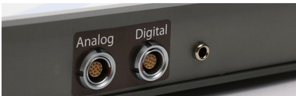
Figure 5: Connectors for Analog and Digital in and output and for the grounding cable (right).
