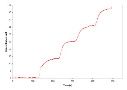
The graph shows a NO sensor response to sequential addition of 12nM of NO. Data points were taken every second. Each of the shown points is the running average of 10 measured data points.
