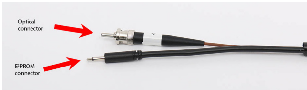
The MicroOptode cable with optical and E 2 PROM Connectors
