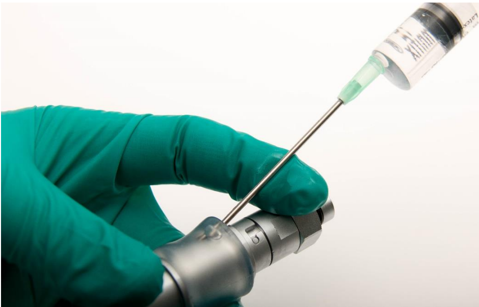
Figure 21: Filling the sleeve with oil and letting the last air escape
