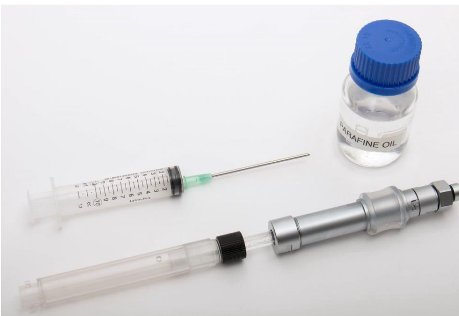
Figure 17: Ready for filling with oil.
