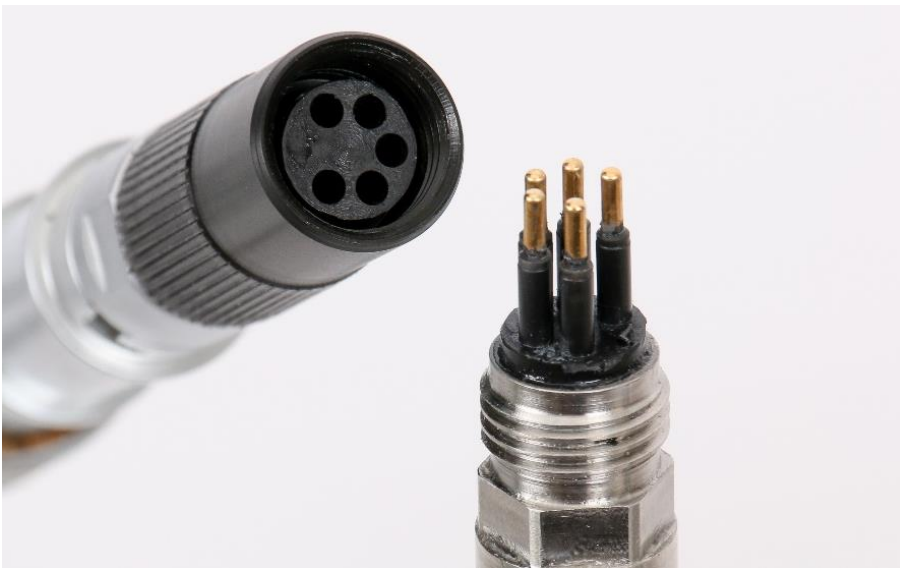
Figure 25: Deep Sea version In Situ UniAmp (right) and UniAmp connector (left).
