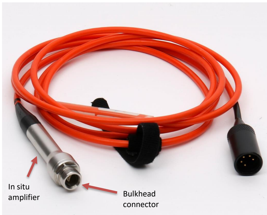
Figure 1: Shallow water In situ UniAmp amplifier.
