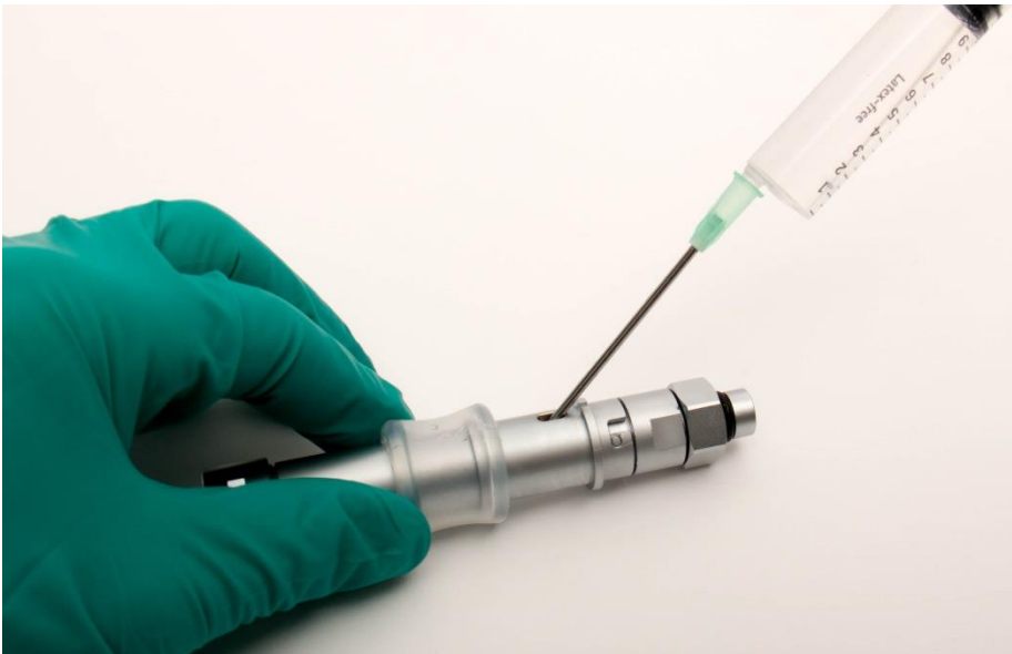
Figure 18: Injecting oil into the UniAmp connector body.
