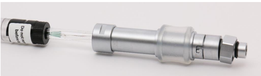
Figure 15: Microsensor with In Situ UniAmp Connector mounted
