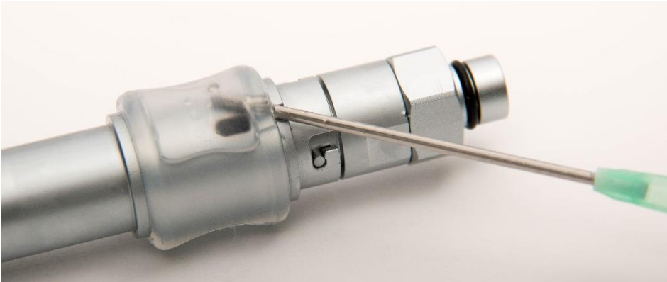
Figure 20: Filling the cavity under the sleeve with oil
