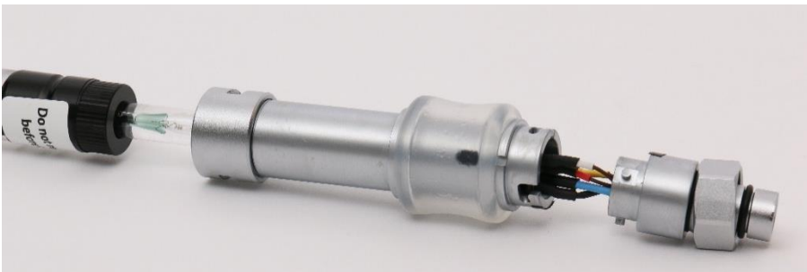
Figure 14: All connections have been made and the sensor must be gently pulled away from the connector body and the cables and the plug must be pushed into the body.
