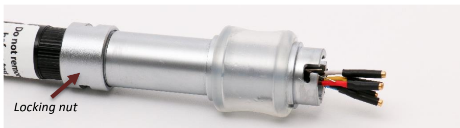
Figure 12: Microsensor inserted in the connector body with the cables and connectors extending.
