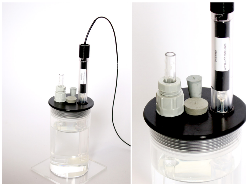
Figure 1: Calibration chamber with sensor. All extra holes in the lid are closed, and the sensor protection tube is lifted from the bottom of the chamber securing circulation of calibration liquid inside the tube. It is held in place with an O-ring.
