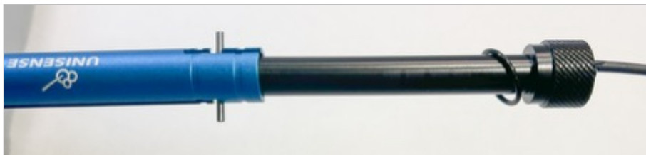
Push the sensor in so that the steel pins engage with the slits in the guide.
