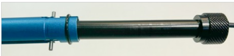
Mount the O-ring in the groove. This ensures that the sensor stays in place.
