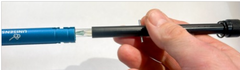
Insert the sensor gently into the blue aluminium guide. The sensor tip should not touch the inside of the guide.
