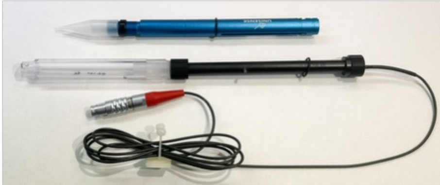
The sensor and the blue aluminium guide before assembly.
