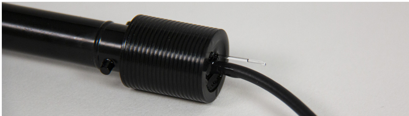
Figure 4: Detailed view of the top of the sensor shaft showing the glass capillary that should be broken off before use.
