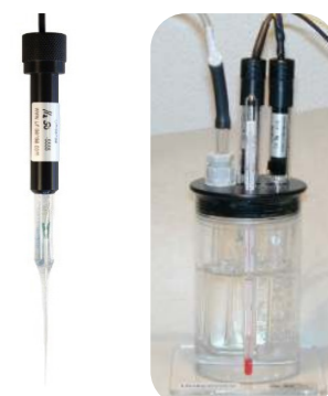
H_2 microsensor CAL300 with microsensors and bubbling with air.
