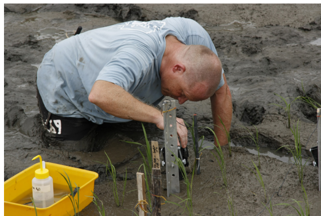
Prof. Ole Pedersen is positioning the sensor tip in the root cortex of the rice plant. Photo: Timonthy D. Colmer
