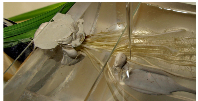
Laboratory setup with double chamber, the sensor is positioned into root cortex. Photo: Ole Pedersen
