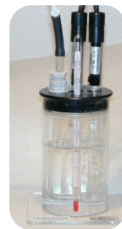
CAL300 with microsensors and bubbling with air.
