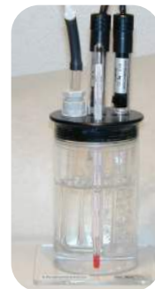
CAL300 with microensors and bubbling with air.
